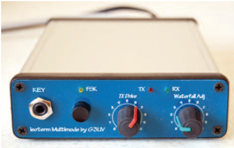
**ISOTERM MULTIMODE.** Isoterm Multimode is very similar to the Multicon USB, but with a few notable differences. First, it has an RS232 interface, so if you are using a modern laptop you will need an RS232/USB converter. I tested it with a cheap model bought off eBay and it worked fine. After all, all it has to do is key the transmitter.
